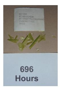
Following its ageing process of 696 accelerated ageing hours (calculated to around 15.2 months at 20°C), the green PE stretch film sample containing Reverte<sup>™</sup> can be seen to have lost all of its significant physical properties, is exhibiting extreme friability and breaking up when handled.
